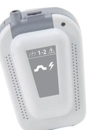
A POD stim/bio is a mobile unit for stimulation and biofeedback, which communicates with the central unit wirelessly. Each POD stim/bio has two stimulation channels and two biofeedback channels
